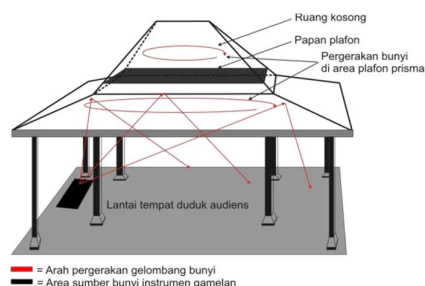
Figure 1. Schematic of the movement of sound waves in the ceiling and roof board area (Santoso, 2018)
