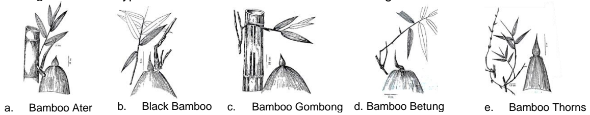
Figure 1. Sastrapradja, Types of Bamboo as Building Materials, 1977, Drawing. Source: Beberapa Jenis Bambu
