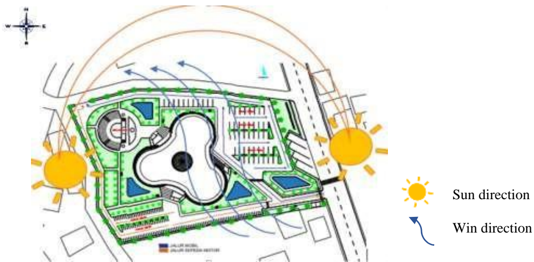
Figure 1: The concept of lighting and ventilation
