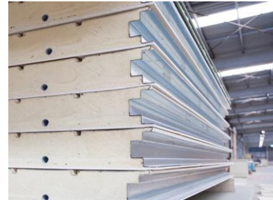
Figure 14. Sandwich panel wall/partition material Source: Google
